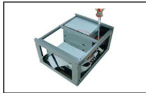
② Dismantle the HD Bracket
