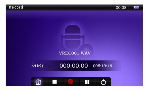
The recording screen will display the name of the file being recorded (VREC001.WAV in the example above) as well as the length of the current recording and the maximum amount of recording time left.
