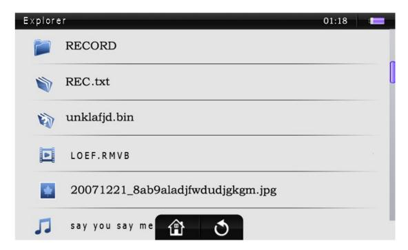
This screen will display only 6 files at a time. If you have more than 6 available, touch the screen and slide your finger up to scroll the screen. Tap the file you wish to access, and it will automatically enter the appropriate mode and begin playing the file.
