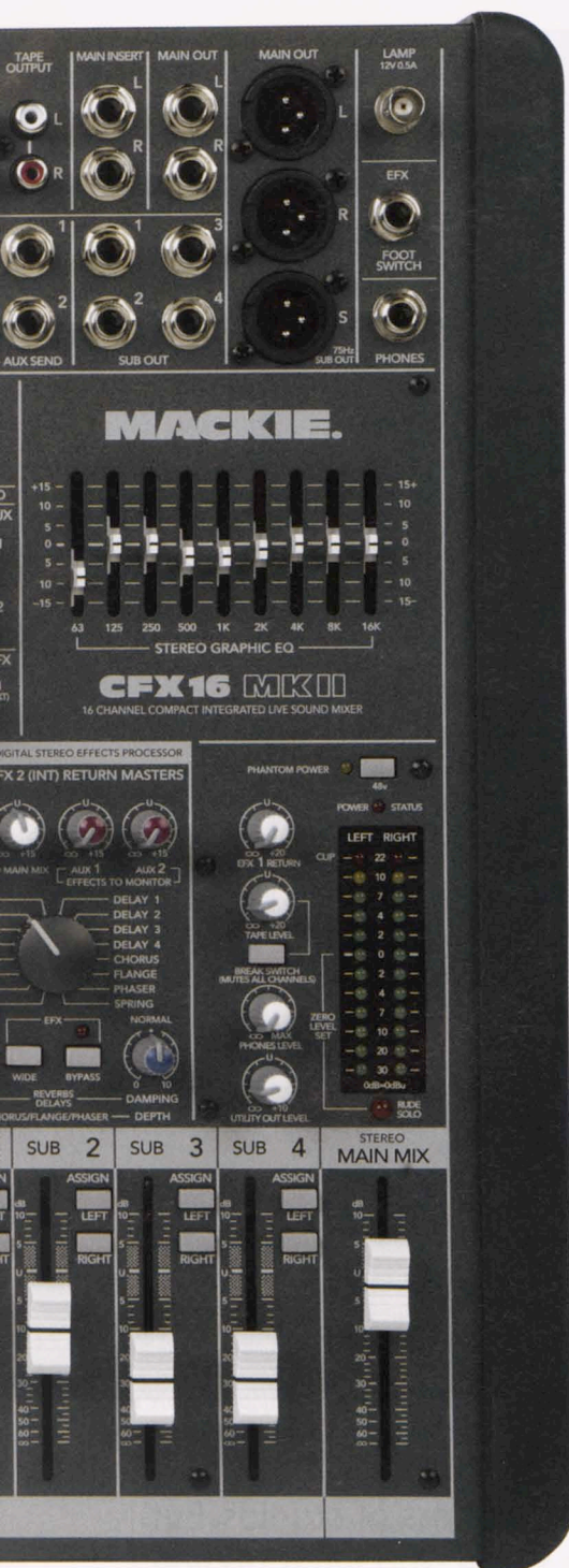
▶ The 'master' connections panel, which includes the remaining ins and outs, plus a BNC lamp socket and a socket for connecting a footswitch to bypass effects.
