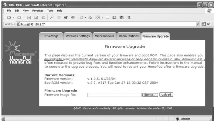
For tech support service, it is often needed to know which versions of Firmware and Boot ROM you have installed in the HomePod. The versions info is displayed in the format of a version number followed by a date time, as below:
