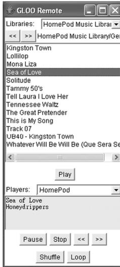
The “Players” field in the bottom half of the window lists all the HomePods located on the network. Select one from the list that you wish to control. The “Libraries” field on top of the window is a pull-down menu listing the available Audio Server on the network. Use the buttons to navigate the list or play and stop songs as you would control the HomePod using the physical HomePod unit.
