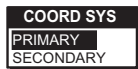
Figure B. You can choose from LAT/LON, UTM, TD, OSGB, Irish, Swiss, Swedish, Finnish, German, French, MGRS and User Grid.
