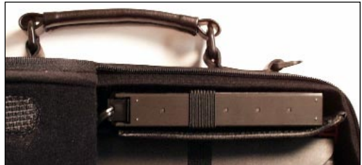
Correctly Installed Battery
