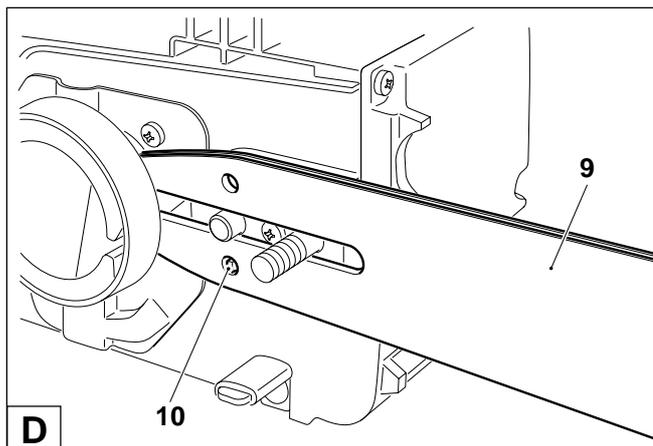
Position the guide bar (9). Make sure that the pin (10) of the chain tightener is in the hole on the guide bar.
