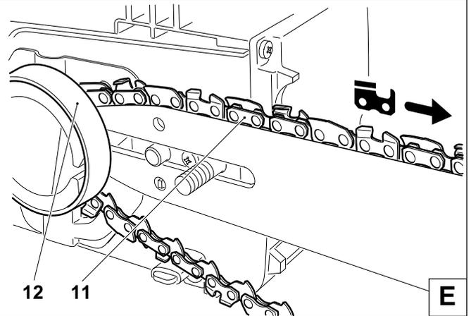
Lead the chain (11) around the sprocket nose (13) of the guide bar.
