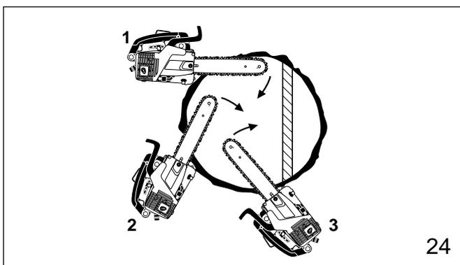
For the sectioning method (fig. 24) make the first cut with the guide bar fanning in toward the hinge. Then, using the bumper spike as a pivot, reposition the saw for the next cut. Avoid repositioning the saw more than necessary. When repositioning for the next cut, keep the guide bar fully engaged in the kerf to keep the felling cut straight. If the saw begins to pinch, insert a wedge to open the cut. On the last cut, do not cut the hinge.
