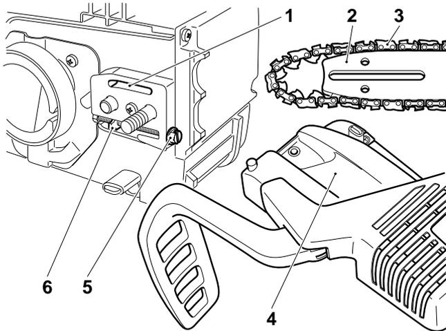
Remove the sprocket guard (4) (see "PUTTING INTO OPERATION" A-B) and use a brush to clean out the interior, especially the area around the brake band.
