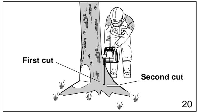
If the tree has large buttress roots, cut into the largest buttresses vertically first (horizontally next) and remove (fig. 20).
