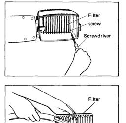
Hose the filter with clean water to remove any dust from it. Be careful not to damage the filter with a brush, stick or the like. Never perform this step near any source of electricity.
