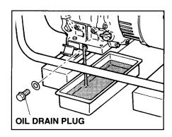
Use fresh and high quality lubricating oil to the specified level as directed on page 6. If contaminated or deteriorated oil is used or the quantity of the engine oil is not sufficient, the engine damage will result and its life will be greatly shortened.
