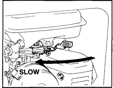
2. Keep depressing the STOP BUTTON until the engine stops. Do not stop the engine suddenly when it is running at high speed.
