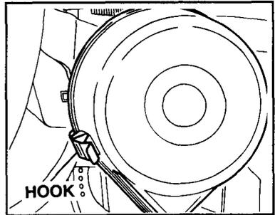
(b) Inner element: Wash the element with kerosene, then soak it in mixed oil (Kerosene (3): Engine oil (1)). Drain the mixed oil.
