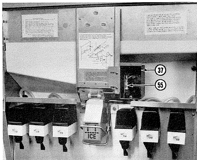
37. Electrical Box Switch 55. Switch/Actuator Pilot Duty
