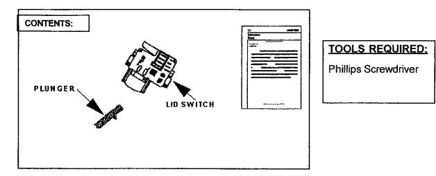
The purpose of this instruction is to inform you of changes made to the switch, making the switch no longer adjustable. The lid switch mechanism is designed to shut off the machine if the lid is lifted no more than 1-7/8" and will allow the machine to start when the lid is less than 1/4" high. The plunger is only used with Atlantis washers.
