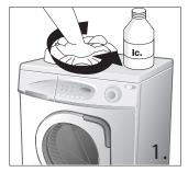
1)Position the unit on a level surface, capable of supporting the entire weight of the dryer. Remember that the unit will be heavier when it is fully loaded. Clean the surface where the stacking kit is going to be installed. Place the mounting bracket on the Washer as indicated.
