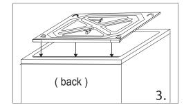
3) Put back edge of stacking kit to back mold line of washer's top cover and tighten the screw.
