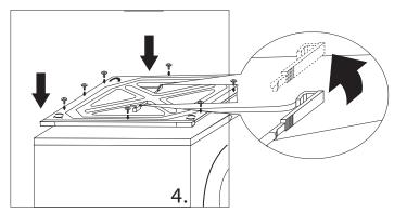
4) Install all 7 screws provided with a power drill and tighten the stacking kit to the unit base securely.
