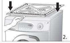
2) Remove the 2 plastic covers (shown in figure 6) attached to the middle of the stacking kit, and save these for later use. Remove the double back tape and firmly attach the stacking kit the top of the washer to assure the proper seal.
