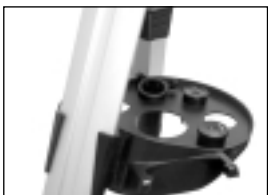
Fig. 5 Attach tray to the tripod:
