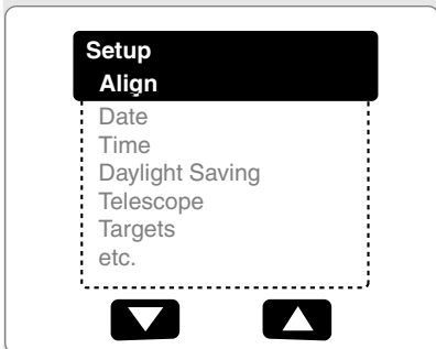
Fig. 26: Menu options display on the second line. Use the Scroll keys to move up or down through the list of options. Press ENTER to select the desired option.
