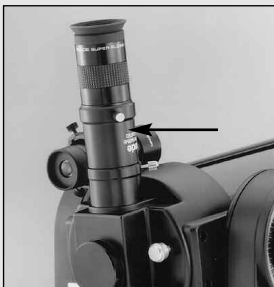
Fig. 35: Use the #126 2x Barlow Lens to double the magnification of the eyepiece employed.
