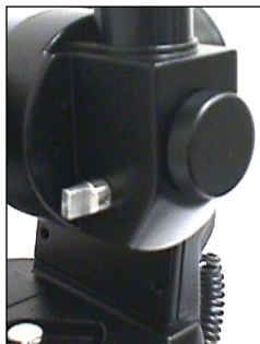
Fig. 2a: Flip mirror control in the "up" position.
