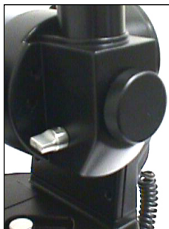
Fig. 2b: Flip mirror control in the "down" position.
