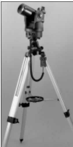
Fig. 30a: The #883 Deluxe Field Tripod shown with an ETX-90EC Astro Telescope, set up in the Alt/Az configuration (tripod head locked at 90°), for terrestrial applications.
