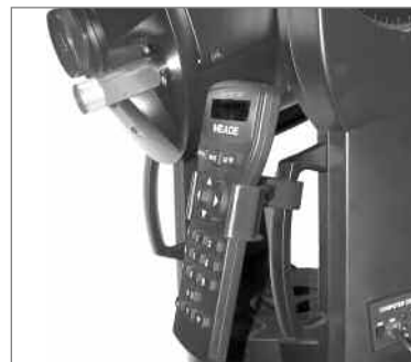
Fig. B: Handbox holder attached to fork arm handle. Adjust holder to a convenient tilt.
