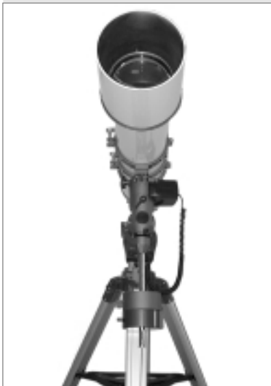
Fig. 16b: The polar home position, front view.
