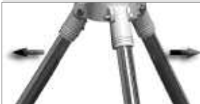
Fig. 3: Spread out the tripod legs. (See next page.)
