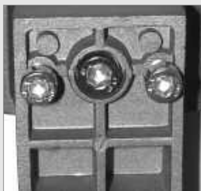
Fig. 47: Cradle adjustment screws.
