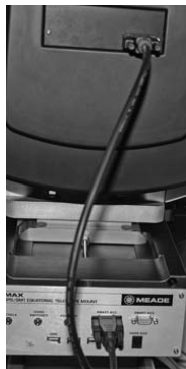
JUMPER CABLE BETWEEN OTA AND SADDLE PANEL (may use either of the Smart Accessory ports)
