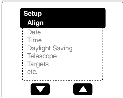
Fig. 29: Menu options display on the second line. Use the Scroll keys to move up or down through the list of options. Press ENTER to select the desired option.
