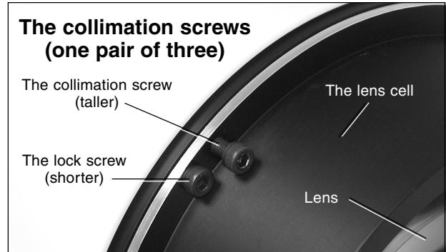
the shorter of the pair is the lock screw that holds the proper collimation after adjustment. Be sure to adjust only one set of collimation screws at a time. Loosen the lock screws before attempting to turn the collimating screws. Make only small changes at a time (turning the collimating screw only a fraction of a turn and checking to see the results before turning further).
