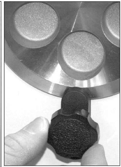
Fig. 18: Tighten the tension adjustment bolt as necessary.
