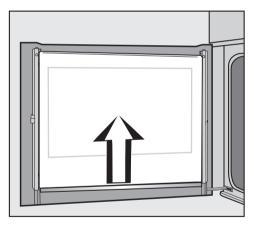
Lift the metal seal from its retainers.
