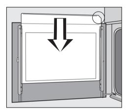
Fit the first of the middle panes into the aluminium trim behind the screw heads.
