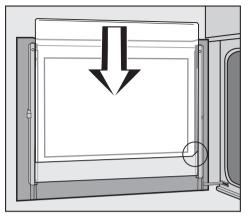
Fit the second pane in the aluminium trim behind the screw heads. The more angled corner must be positioned at the bottom right-hand side.
