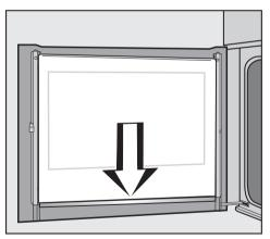
■ Fit the metal seal at the bottom on the retainers in front of the panes.
