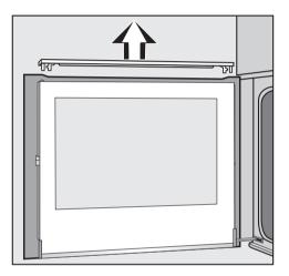
Pull the cover trim up off the door. The inner door pane will tip slightly forward as it slips out of the groove in the cover trim. This is quite normal.
