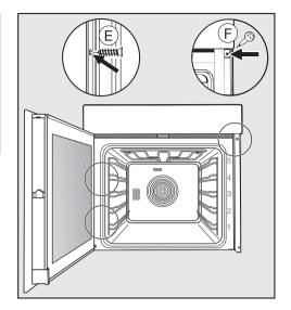
Open the oven door and secure the oven to the side walls of the housing unit as illustrated.
