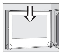
Fit the inner door pane into the plastic runners. The drip channel will slip between the plastic runners as you do this.
