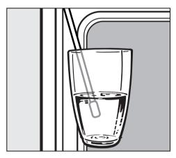
Hold a container with the quantity of water specified under the tube as shown. Start the water intake process with "OK". The amount of water required will be drawn up into the oven. As the water is taken in, bars will appear in the display. The amount of water specified will be more than the amount which is actually needed which means that some of the water will remain in the container as not all of it will be drawn up into the oven.
