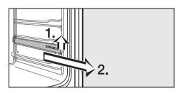
Lift the FlexiClip runner up at the front and pull it out along the rail of the side runner.
