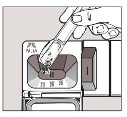
The horizontal marks in Compartment II indicate levels of approximately 1  $^{1}/_{4}$ , 1  $^{3}/_{4}$  and 2 tablespoons (20, 25 and 30 ml) respectively.
