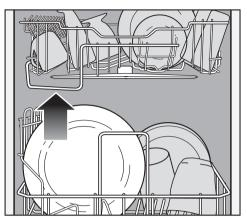
The guide at the front of the upper basket determines the maximum height for items placed in the lower basket so that the middle spray arm is not blocked. Various removable inserts are available for the lower basket to accommodate special items to be washed.
