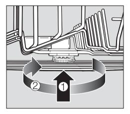
■ Lift up the **middle** spray arm, ①, to engage the ratchet and unscrew the spray arm, ②. Remove the lower basket.
