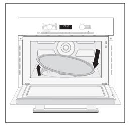
■ Remove the turntable, and wash in the dishwasher or by hand.
