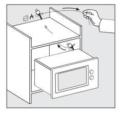
Push the microwave oven into the niche and pull the cable with the plug through the back of the unit.
