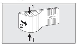
Press the sides of the lamp cover inwards (1), disengage the cover (2) and unclip it at the rear. Replace the lamp.Lamp specification:220 - 240 V, max. 25 W, E 14 fitting.
