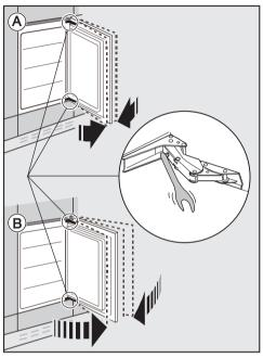
To do this, use the allen key supplied to adjust the door hinges.
