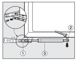
■ Open the hinges, and loosen the screw in mounting ①.
