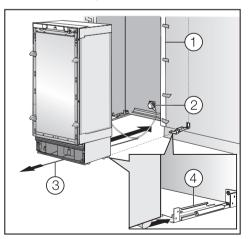
To protect the corners of the installation space, attach the supplied edge protector ① on both sides with adhesive tape. Plug the appliance into the power outlet <sup>(2)</sup>.
