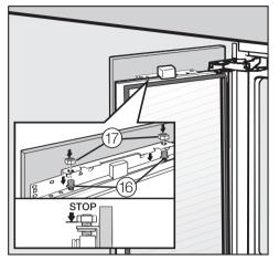
Open the door and hang the custom door with the mounting frame over the threaded bolts <sup>(16)</sup>.
