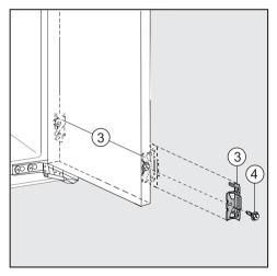
Secure fixing brackets ③ (supplied) to the appliance doors by screwing a hexagon screw ④ into the pre-drilled holes.
