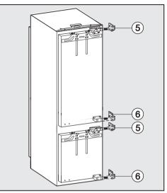
Clip spacers (5) onto the top hinges and spacers (6) onto the bottom hinges.
