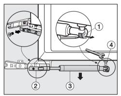
Using a screwdriver, carefully push tension spring ① outwards.
