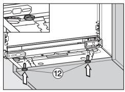
■ Screw in adjustable feet <sup>12</sup> completely.
