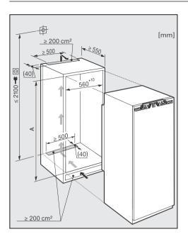
Before installing the appliance make sure the housing unit is the correct size. Specified ventilation gaps must be maintained in order to ensure that the appliance functions correctly.
