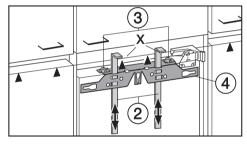
■ Remove the nuts ③ and detach the mounting frame ④ together with the fitting aids ②.
