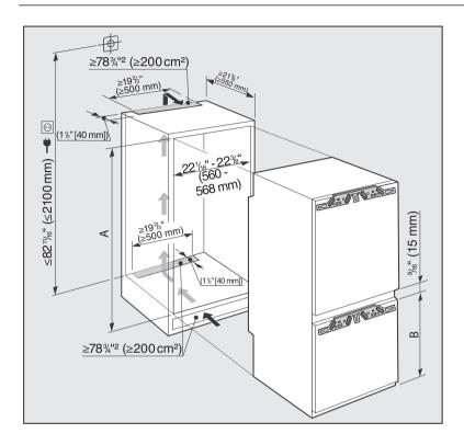
Before installation, make sure that the cabinet space matches the required dimensions. The specified measurements for the ventilation openings must be adhered to in order to ensure the proper functioning of the appliance.
