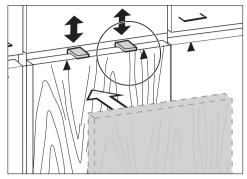
**Tip:** Slide the fitting aids ② and the cabinet front up to the height of the adjacent cabinet unit doors.
