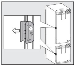
■ Open the appliance door and remove the red transport clips ① (depending on model).
