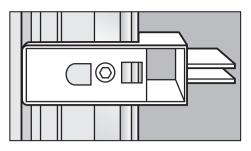
Do not remove the installation supports from the appliance door. They will be used later in the installation niche.
