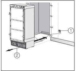
To protect the corners of the installation space, attach edge protectors where needed (not included).  Plug the appliance into the power outlet ①.
