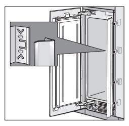
Insert the cover strip into the space between the appliance and the side panel.
