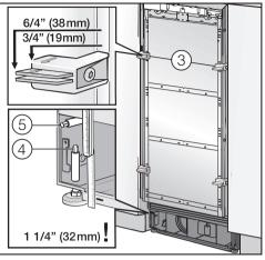
The installation aids 3 on the appliance door have been designed for custom door thicknesses of 3/4" (19 mm) and 1 1/2" (38 mm).
