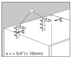
Risk of tipping The installation niche must be securely attached to the wall behind it. This is the only way the appliance, which is later secured in the niche, can be prevented from tipping!
