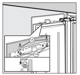
■ Open the door and hang the custom door with the mounting frame over the threaded bolts ④.
