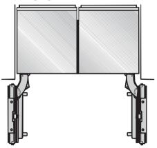
If the appliances are installed directly next to each other (without a partition), they need to be attached together using the "Merging Kit".
