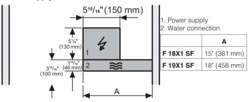
Install a pressure limiting device and water hammer arrester for inlet water pressures exceeding 80 psi.(Refer to Uniform Plumbing Code, Sections 608.2 and 609.10) Never install or operate where inlet water pressure may exceed 120 psi.
