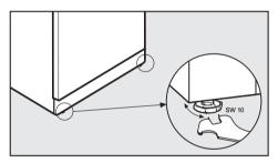
Align the feet using the spanner supplied.
