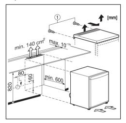
When placed under a worktop run it is essential that adequate ventilation is provided at the rear of the appliance. A ventilation gap of at least 140 cm<sup>2</sup> must be made in the worktop.
