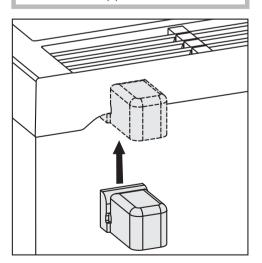
Fit the wall spacers onto the back of the appliance on the top left and right.
