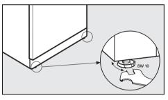
To align the appliance, adjust the feet using a suitable spanner.
