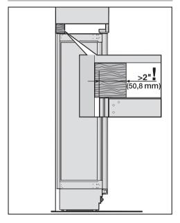
Cut a wooden beam (cross section min. 3" x 4" [75 mm x 100 mm] to the required length). The length is equal to the width of the installation niche.
