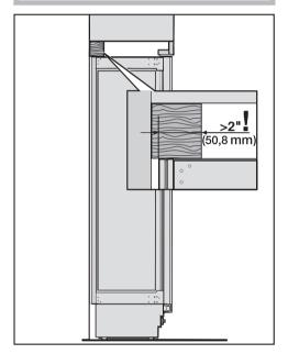
Cut a wooden beam (cross section min. 3" x 4"
