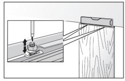
■ Tighten the nuts on the adjusting rail. This will correct the side alignment of the door.
