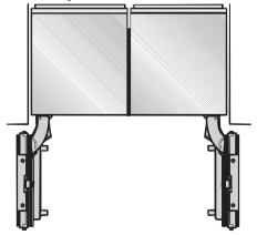
If the appliances are to be installed next to each other without a partition wall between them, they will need to be joined together using the side-by-side installation kit.
