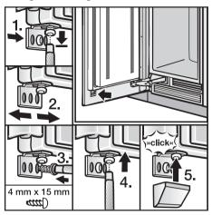
The fixing brackets are used to secure the furniture front to the bottom of the appliance door.
