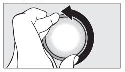
■ Turn the lamp cover anti-clockwise to remove it.
