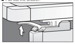
■ Raise the snap fittings on both sides and lift the drawer out.
