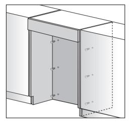
screw the back panel directly onto the wall behind in a number of places. Use suitable wall plugs/fixing screws for the type and material of the wall. For a unit without a back panel
