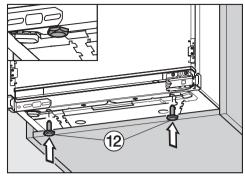
■ Screw in adjustable feet ② completely.
