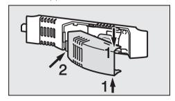
Grasp the lamp cover at the top and at the bottom (1), and pull it forwards to remove (2).
