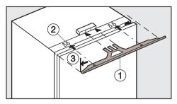
Slide cover strip ① into the holder as shown, with the bumps facing downwards. The bumps will fit into keyhole slots ②. The cover strip is then flush with the side of the appliance on which the door is opened ③.
