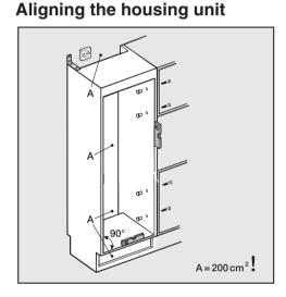
Before installing the appliance, the housing unit must be carefully aligned using a spirit level. The housing unit corners must be at right angles, as otherwise the appliance furniture door will not align correctly with the 4 corners of the unit. Align the furniture door with the hinges.
