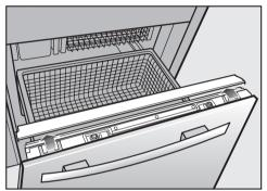
■ To remove the stainless steel front, loosen the two nuts and remove the cover strip.
