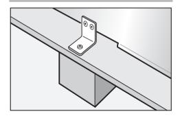
Loosen the bracket that holds the appliance to the pallet. ⚠ Caution! The appliance is no longer secured and may be unstable.
