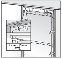
If there is no way to attach the top of the appliance, it can be attached to the sides of the installation niche.
