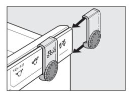
Slide the markers onto the guide runners on the edge of the drawers.
