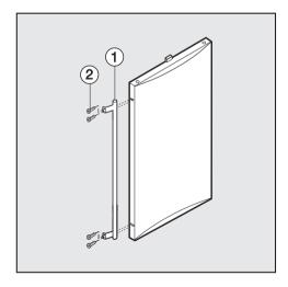
■ Secure handle ① to the holes in the door using the screws marked ②.
