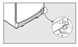
■ To align the appliance adjust the feet using the spanner supplied.
