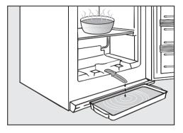
Place a container in front of the appliance to collect the defrosted water.
