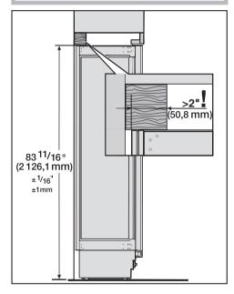
Cut a wooden beam (cross section min. 29 <sup>1</sup>/<sub>2</sub>" x 39 <sup>3</sup>/<sub>8</sub>" [75 cm x 100 cm]) to the required length. The length is equal to the width of the installation niche.
