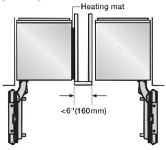
For instructions on how to install the heating mat please refer to the instructions included in the "Merging Kit". The "Merging Kit" can be obtained from Miele.
