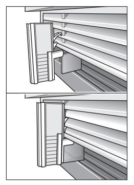
Clip the air separator, left and right of the partition, in the exhaust grille. Be sure that it clicks into place and guides the foam partition under the exhaust grille.
