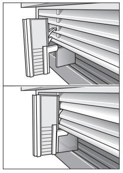
■ Clip the air separator, left and right of the partition, in the exhaust grille. Be sure that it clicks into place and guides the foam partition under the exhaust grille. All plumbing work should be carried out by a suitably qualified and competent person, in accordance with all applicable local and national regulations.
