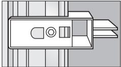
■ Do **not** remove the installation supports from the appliance doors. They will be used later in the installation niche.
