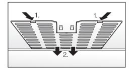
■ Unhook the filter cover, **1.** in each side of the drawer and remove them along with the filters downwards starting from **2**.
