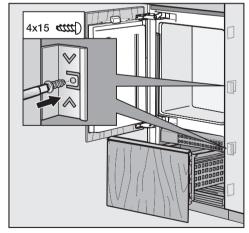
Screw the brackets onto both sides of the appliance, to hold the cover strip.
