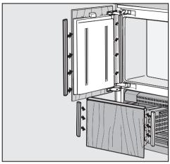
■ To mount the cover strips on both sides of the upper and lower doors, click them into place from bottom to top, into the gap between the appliance door and the custom door.
