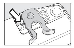
■ Using a screwdriver, remove spring clamp <sup>③</sup> from underneath the door and fit it on the opposite side.
