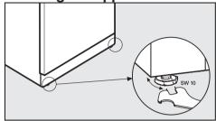
■ **Ensure** that you unscrew adjusting foot ① from the hinge plate until it sits on the floor. Then unscrew the foot by a further 90°.
